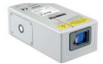
The new DLS-B optical measuring device can measure absolute distances up to 500m with a precision of 1.5mm. It represents a cost efficient solution even at extreme environment temperatures as low as -40°C. Serial, analogue and digital interfaces are standard features enabling you to easily connect the DLS-B to a control system (SPS, IPC or PC). The device measures distances on natural and reflective surfaces and determines positions of objects with difficult access or high surface temperatures.
